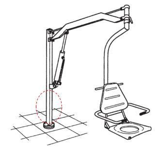
NOTE: Do not continue to use the Dipper hoist if any structural damage/deformation of the mast framework is detected after conducting the safe working load 140kg test.
