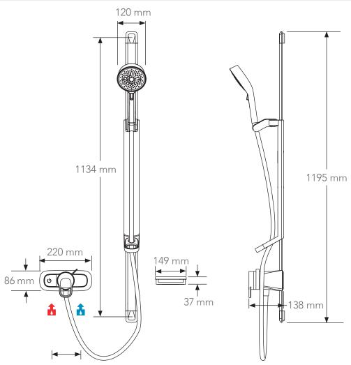
110 - 155 mm Adjustable Pipe Centres - Rear Entry Pipework Only
